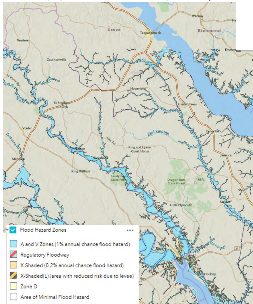
Flood Hazard Zones in King & Queen County (Virginia Flood Risk Information System, 2021)
